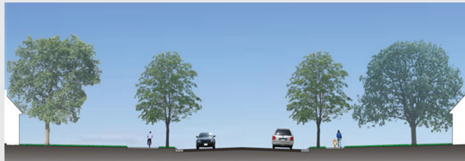
Example of two lane road with center turn lane, addition of boulevards, trail on one side and sidewalks on the other.
