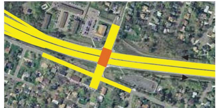
Option 2: Overpass or Underpass
