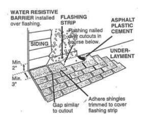
The flashing strip should be bent, using a metal brake, to extend at least 2 in. up the vertical wall and at least 3 in. onto the last shingle course (to the top of the cutout).
